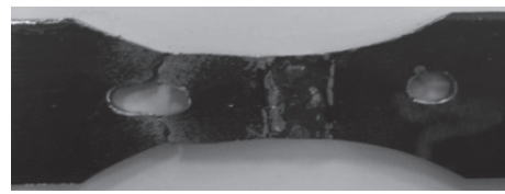
Fig. 7 Specimen with concave sides after testing
